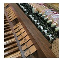
There are five wire connections to each of the 21 stop tablets plus wiring for the stop pistons (those little black buttons below the key board).
