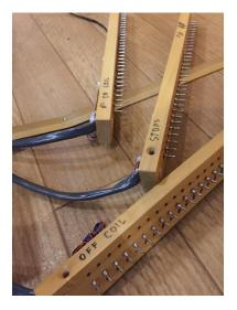
Stop tablet wiring connects to a set of pin boards at the back of the organ console from which the wiring travels beneath the floor connecting to the capture system mounted in the organ case. Each pin serves as a connection point.
