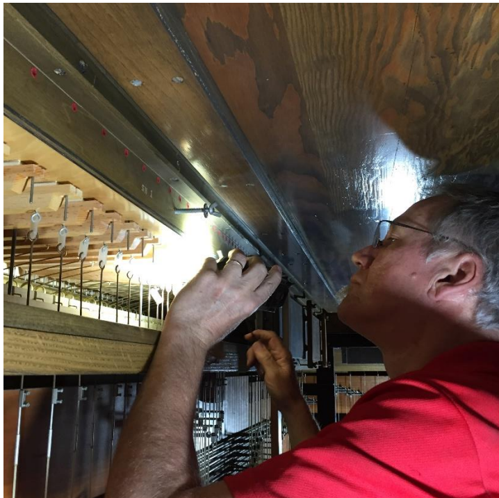
Thomas Rohlf inspects and cleans the pallet valves of the Swell Division of the pipe organ.
