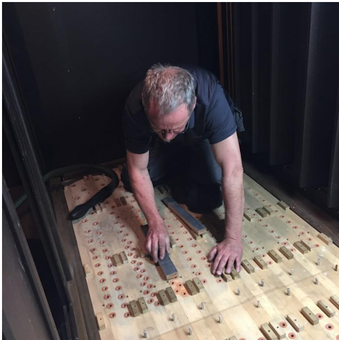
Thomas Rohlfs of Rohlfs Pipe Organ Services sands and levels the vulcanized paper washers placed over the air holes in the top of the wind chest or table of the Swell Division of the organ.
